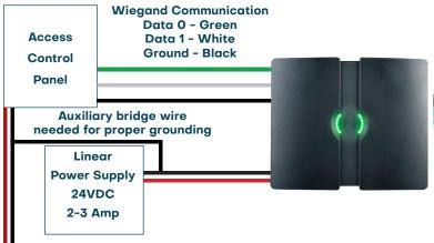
Continuity is created by landing a jumper between the 12v ground powering the access control panel to the 24v ground powering the reader.
